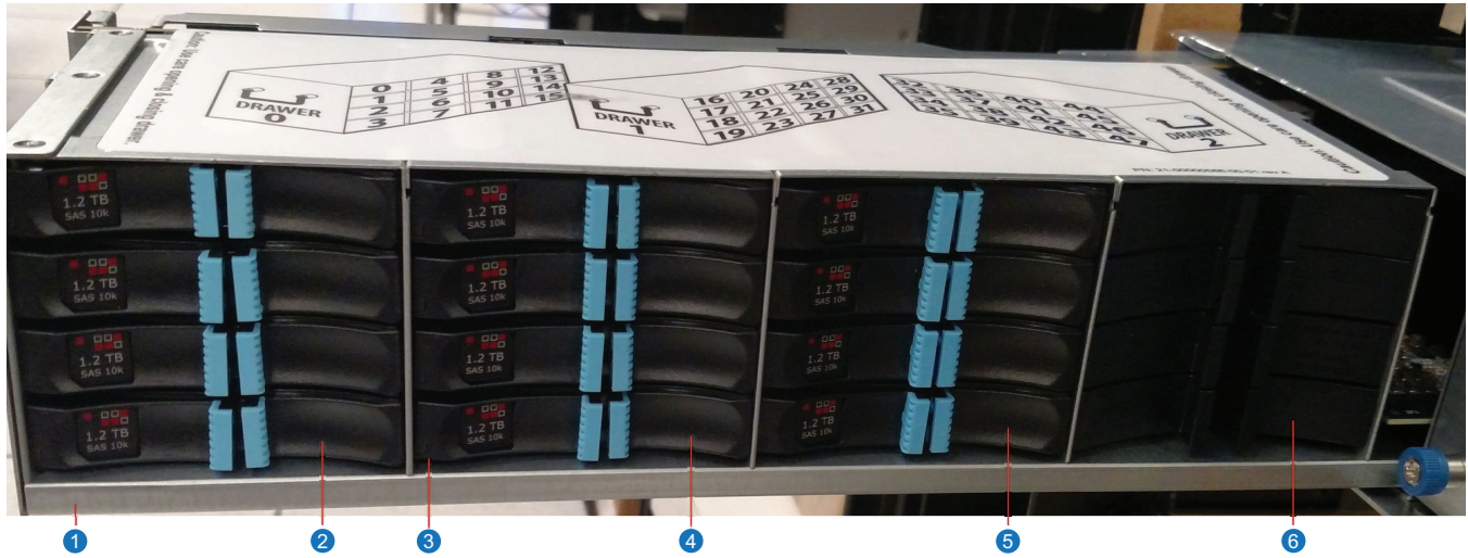
Figure 40: 2U48 Drive Chassis: Sample Drawer Population
