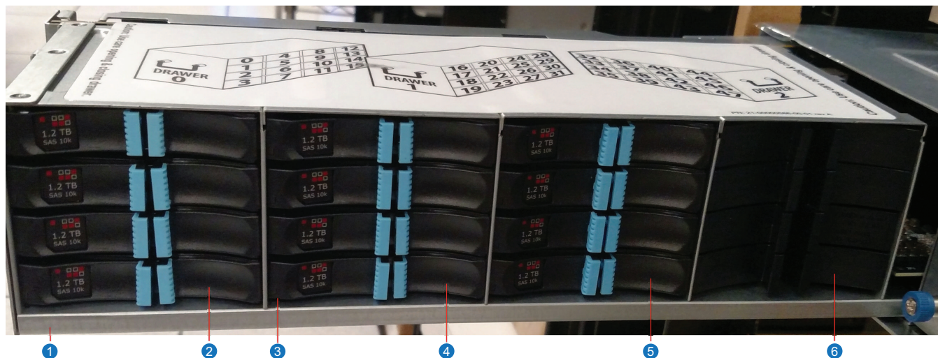
Figure 20: 2U48 Drive chassis: Sample Drawer Population
